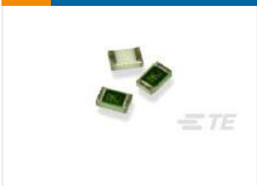
TE Part #2-1614893-0 CPF 0805 19K1 0.1% 25PPM 1K RL
