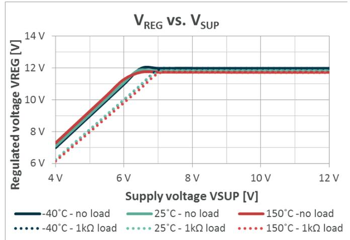
Figure 10-5 MLX83203 Regulated output voltage vs. supply voltage
