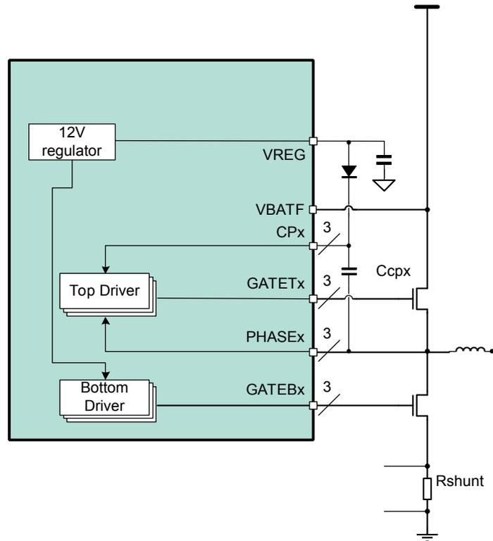
Figure 12-20 Voltage regulator for driver supply - VREG
