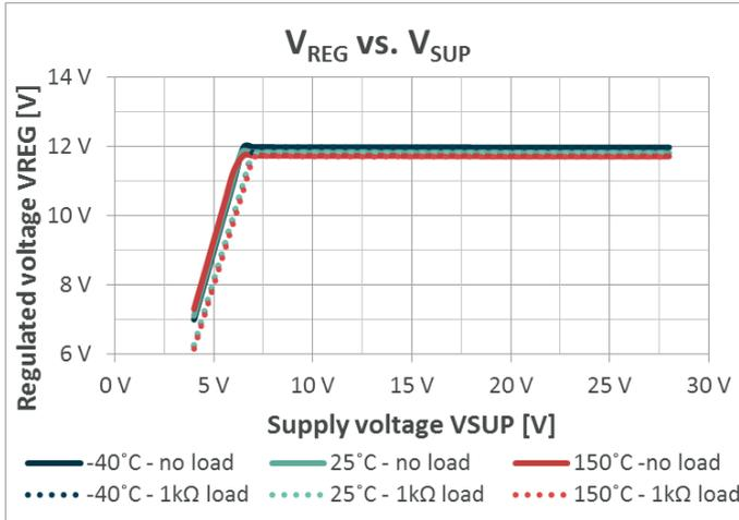
Figure 10-4 MLX83203 Regulated output voltage vs. supply voltage
