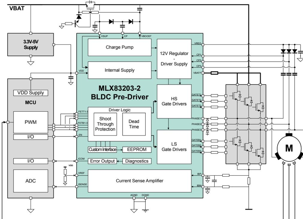
Figure 4-2 Alternative application diagram with reverse polarity N-FET
