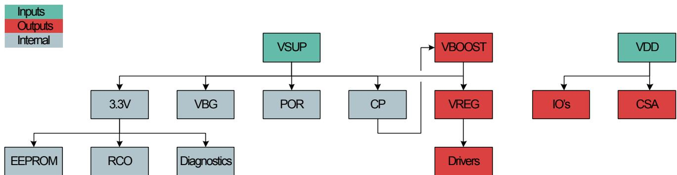
Figure 12-17 Principle organization of the supply system
