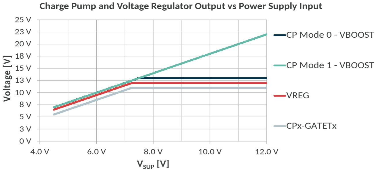
Figure 12-19 Charge pump output and driver supply
