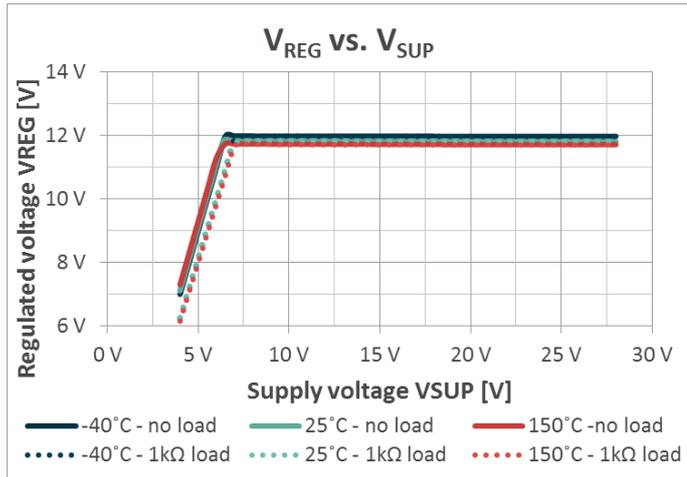
Figure 10-10 MLX83202 Regulated output voltage vs. supply voltage
