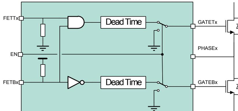
Figure 12-21 Input control logic of the driver stage
