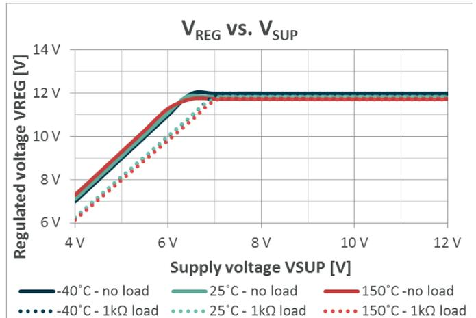
Figure 10-11 MLX83202 Regulated output voltage vs. supply voltage
