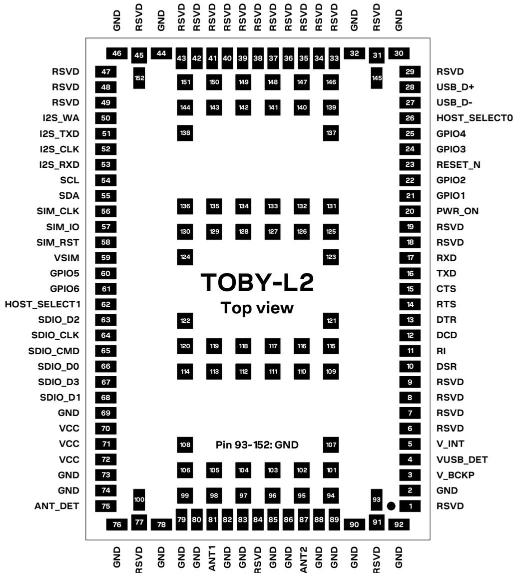
Figure 2: TOBY-L2 series pin assignment (top view)
