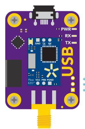
Connect Flow breakout board to the carrier board.
