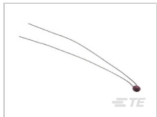
Discrete NTC Sensor Type: **Epoxy Coated NTC Thermistor**Wire Connection: **Open End**Discrete NTC Wire Length: **76 mm**Resistance (at 25°C): **100 kΩ**Beta 25/85 Value: **4261 K**[All DISCRETE NTC SERIES I \(26\)](#)
