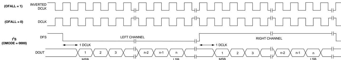
**Figure 11. I<sup>2</sup>S Digital Audio Format**
