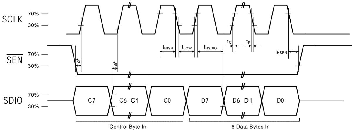
**Figure 6. SPI Control Interface Write Timing Parameters**
