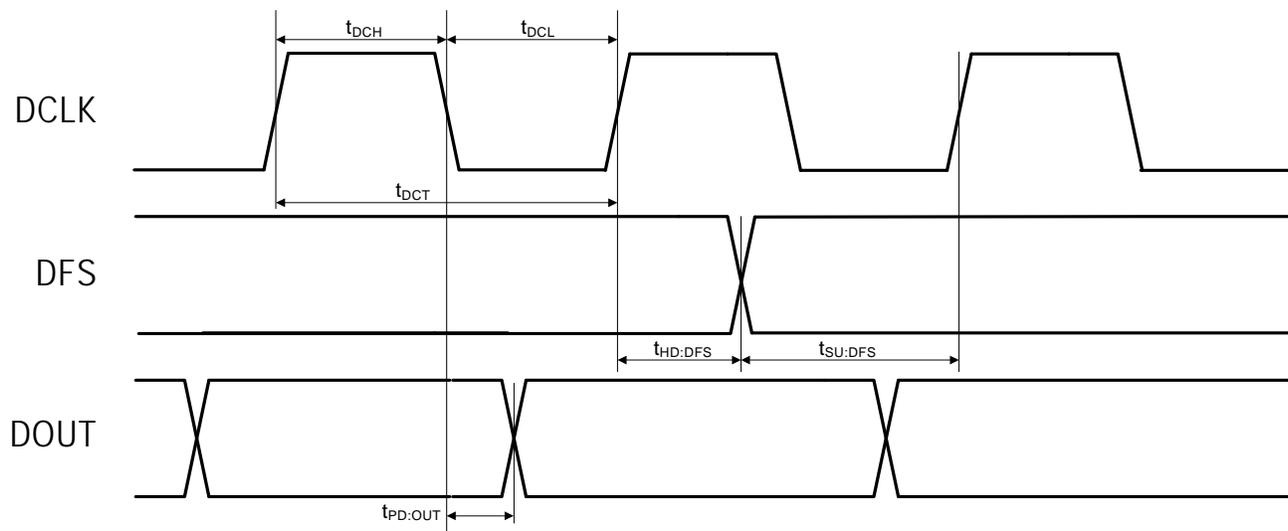
**Figure 8. Digital Audio Interface Timing Parameters, I<sup>2</sup>S Mode**
