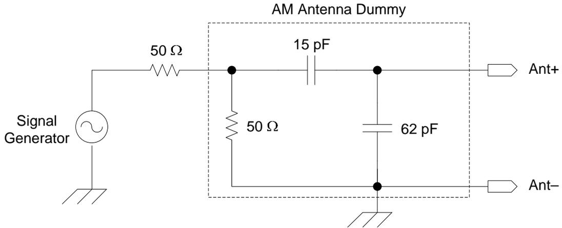
**Figure 9. AM Test Circuit**
