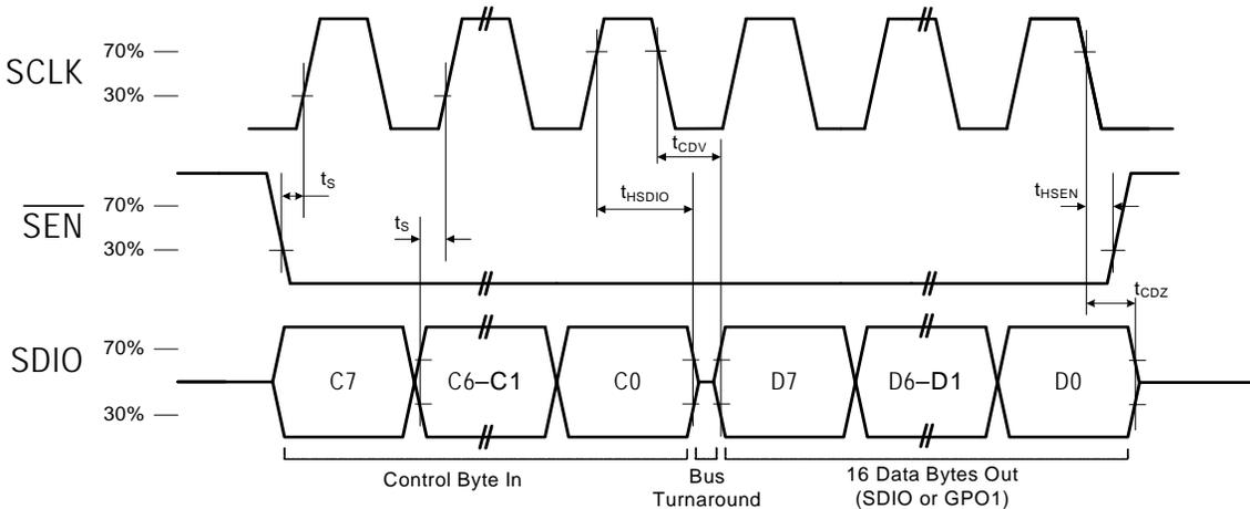
**Figure 7. SPI Control Interface Read Timing Parameters**
