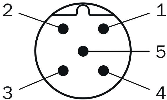
Connector M12, 5-pin, A-coded
