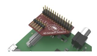
4D Pi Serial Adaptor attached to a Raspberry Pi
