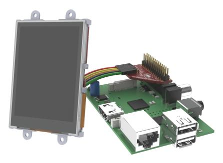
4D Pi Display Module Pack (4D Pi Serial Adaptor is one part of this pack)
