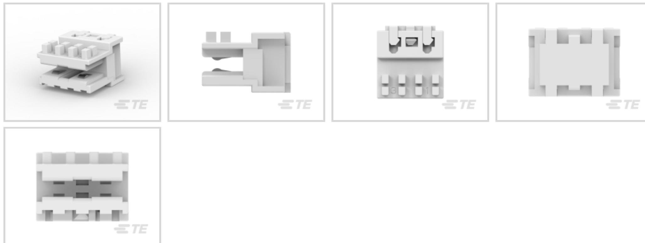
Connector System: **Wire-to-Board**Number of Positions: **2**Centerline (Pitch): **2.5 mm [.098 in]**Termination Method to Wire & Cable: **Insulation Displacement (IDC)**Number of Rows: **1**
