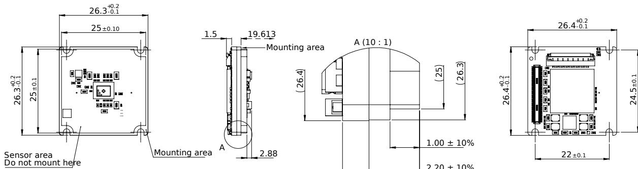
Sensor and electronic components are schematics and vary between models.
