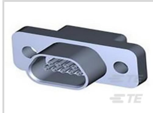
Connector & Housing Type: **Receptacle**Connector System: **Cable-to-Board**Number of Positions: **25**Centerline (Pitch): **1.27 mm [.05 in]**Connector & Contact Terminates To: **Wire & Cable****Features****Product Type Features**
