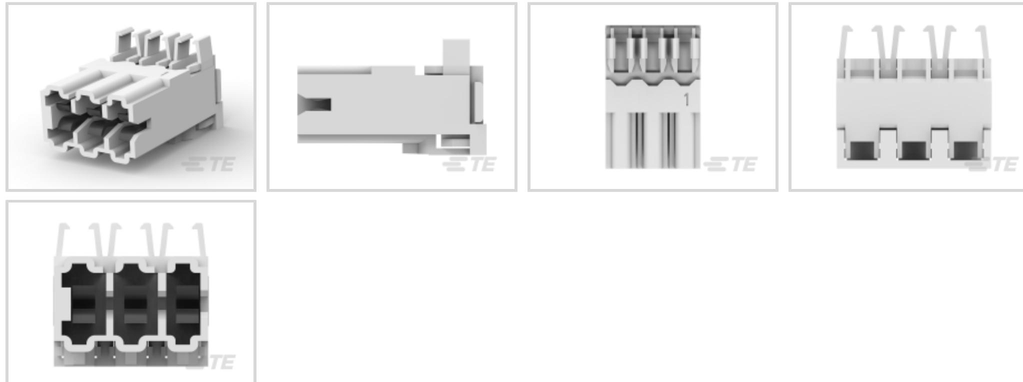
Connector System: **Wire-to-Board**Number of Positions: **3**Centerline (Pitch): **5 mm [.196 in]**Termination Method to Wire & Cable: **Insulation Displacement (IDC)**Number of Rows: **1****Features****Product Type Features**
