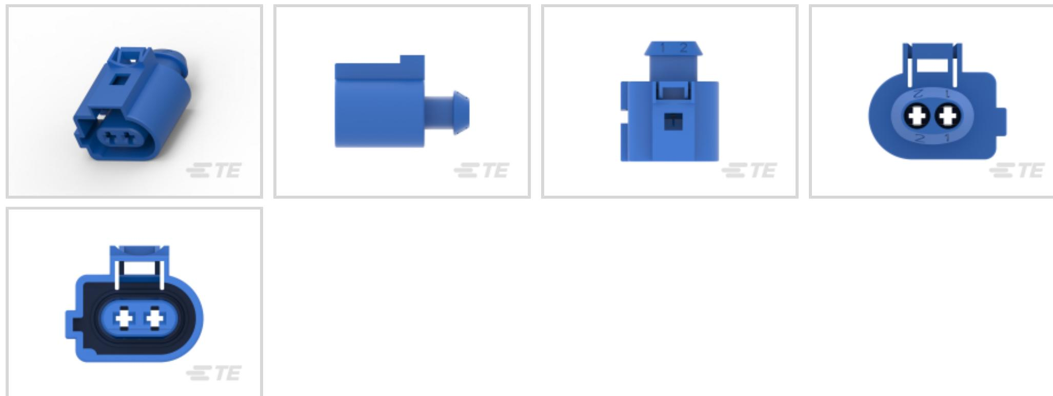
Connector System: **Wire-to-Wire**Number of Positions: **2**Connector & Housing Type: **Housing for Female Terminals**Centerline (Pitch): **6 mm [.236 in]**Sealable: **Yes**[All AMP MCP, SEALED CONNECTOR HOUSING \(172\)](#)**Features****Product Type Features**
