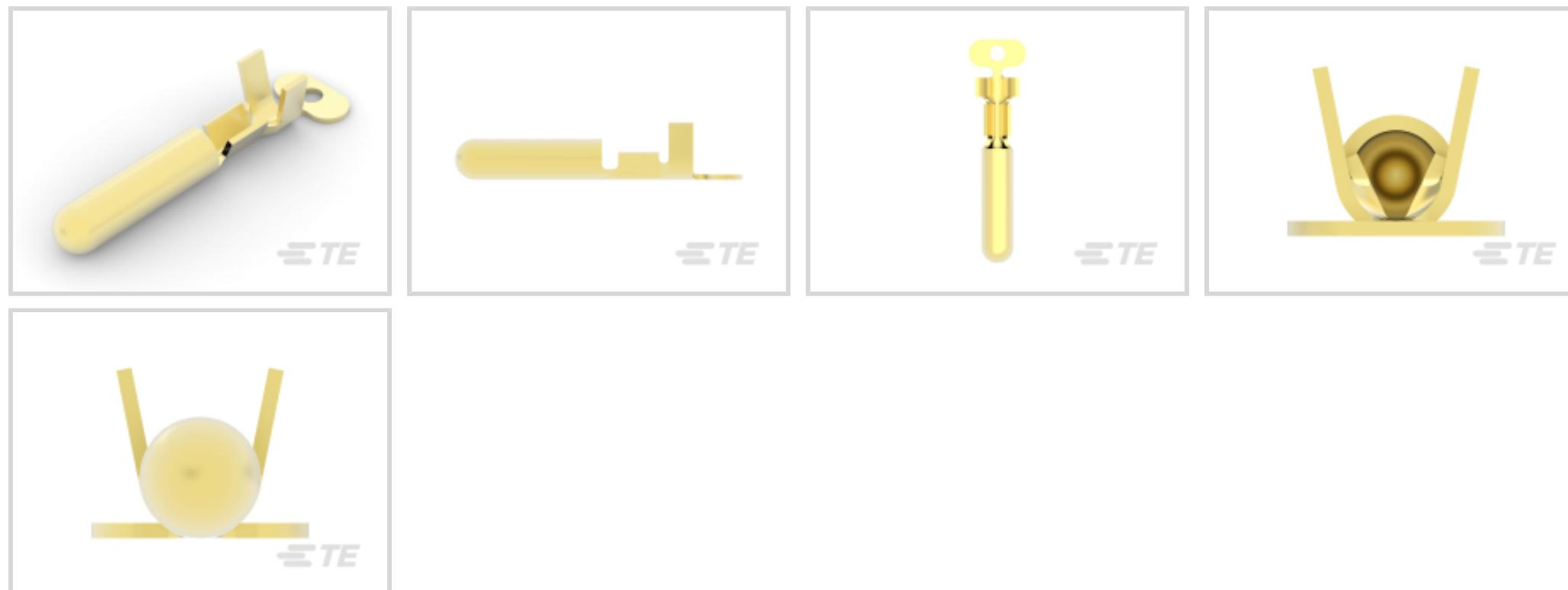
Crimp Wire Terminal Type: **Pin**Mating Pin Diameter: **3.17 mm [.125 in]**Compatible Insulation Diameter Range: **1.52 – 2.62 mm, 2.62 mm [.06 – .103 in, .103 in]**Wire Size: **.2 – .6 mm<sup>2</sup>**
