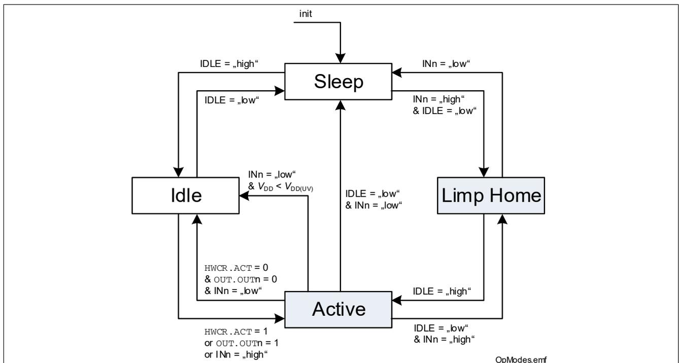
Figure 13 Operation Mode state diagram
