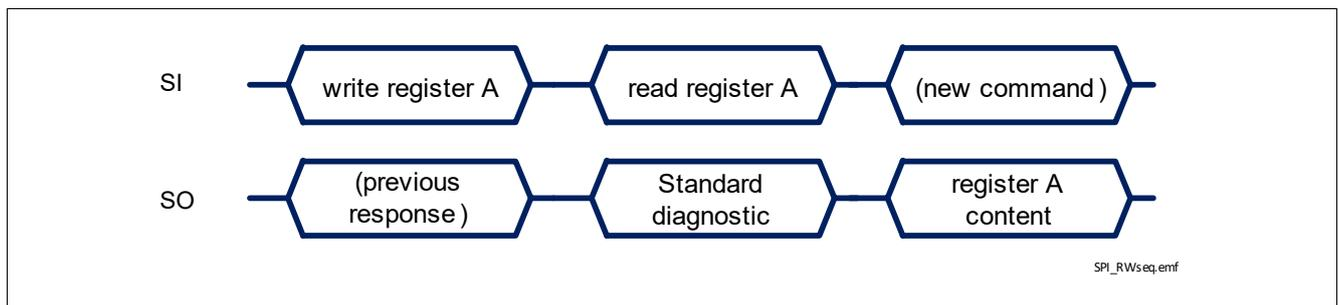
**Figure 32 Register content sent back to  $\mu\text{C}$**
