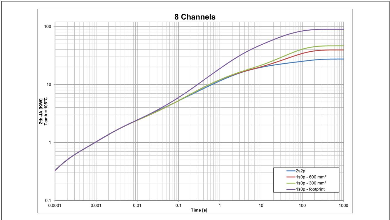
Figure 8 Typical Thermal Impedance. PCB setup according [Chapter 4.3.1](#)
