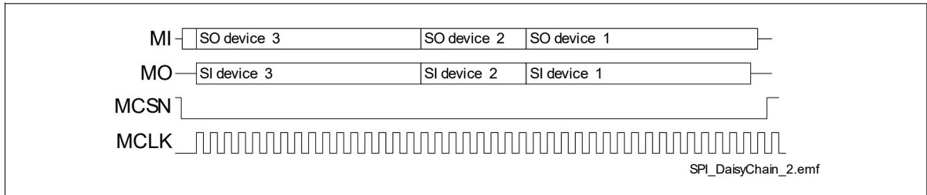
**Figure 29 Data Transfer in Daisy Chain Configuration**
