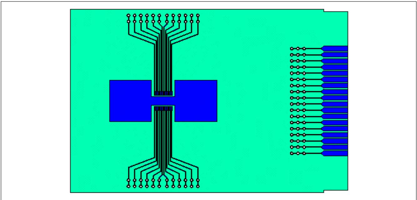
Figure 6 PC Board for Thermal Simulation with 600 mm<sup>2</sup> Cooling Area
