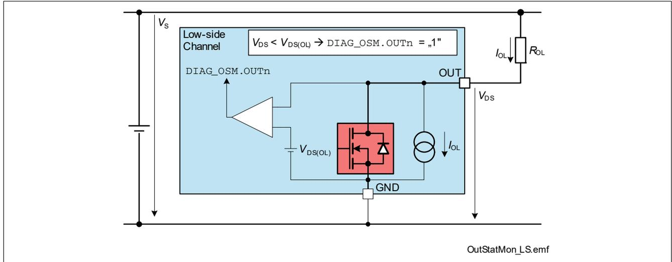
Figure 23 Output Status Monitor - concept (Low-Side channels)
