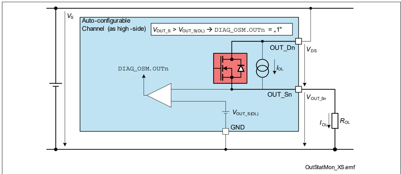
Figure 24 Output Status Monitor - concept (auto-configurable channel as High-Side)
