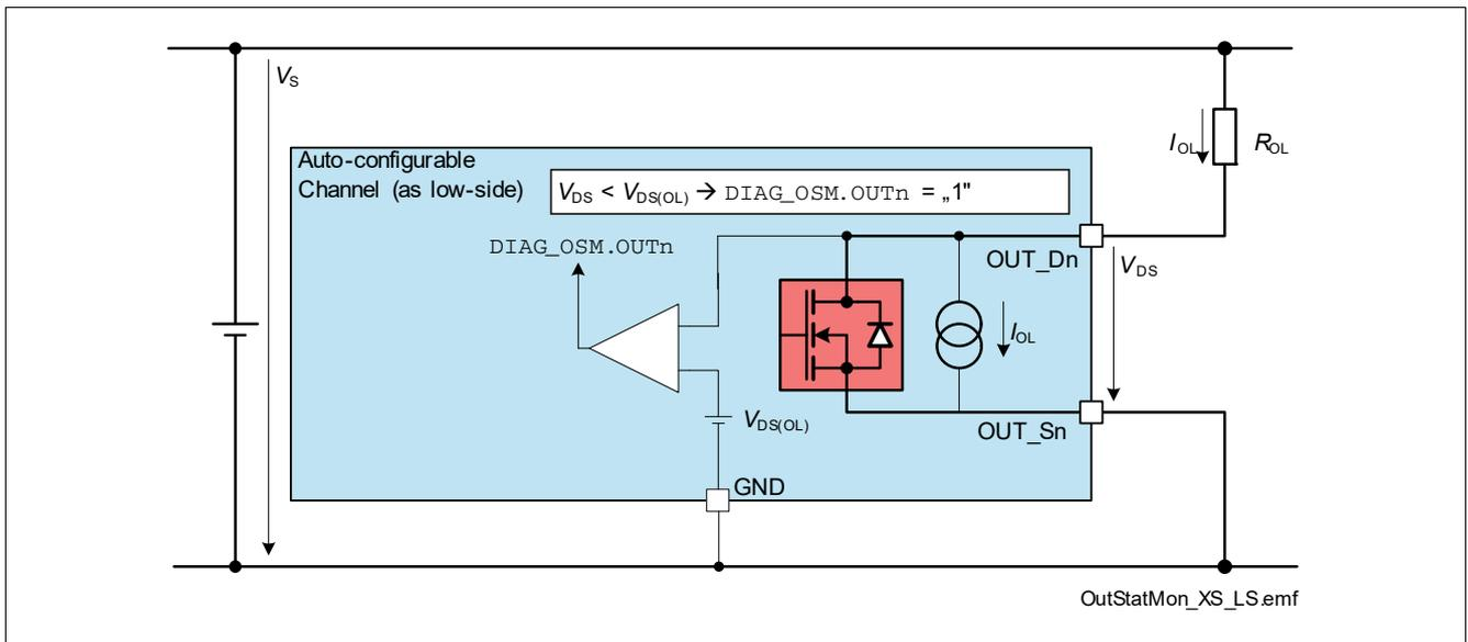
Figure 25 Output Status Monitor - concept (Auto-configurable channel as Low-Side)
