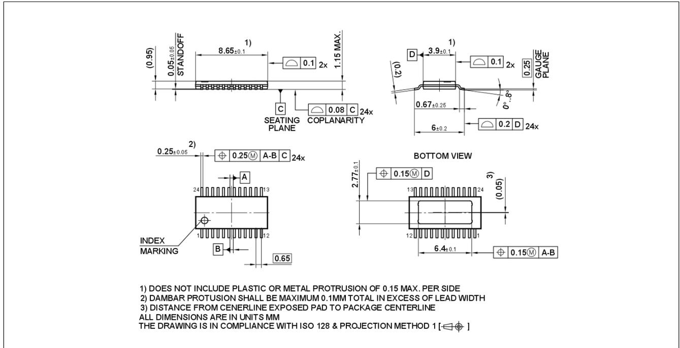
Figure 37 PG-TSDSO-24 Package drawing
