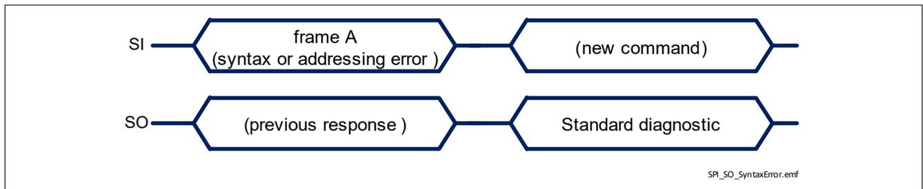
Figure 35 TLE75602-ESD response after a command syntax error
