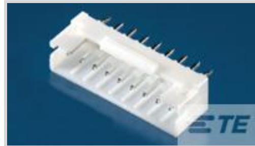
Connector System: **Wire-to-Board**Number of Positions: **11**Number of Rows: **1**Centerline (Pitch): **2 mm [.079 in]**PCB Mount Orientation: **Vertical**[All AMP HPI 2.0 mm Headers \(206\)](#)
