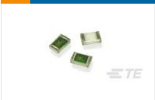
TE Part #1676153-2 RN 0805 10K 0.1% 10PPM 1KRL
