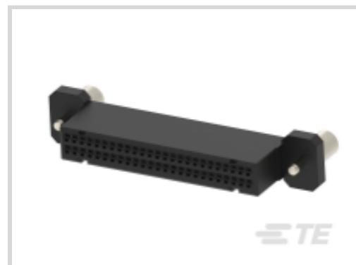
Connector Product Type: **Housing**Connector & Housing Type: **Receptacle**Connector System: **Wire-to-Board**Number of Positions: **50**Centerline (Pitch): **2.5 mm [.098 in]**[All Receptacle and Tab Housing: 2.5 mm Pitch, 250V \(54\)](#)
