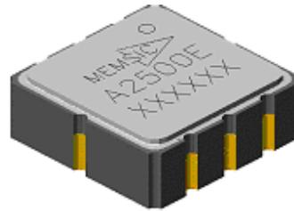
**Note:** The MEMSIC logo's arrow indicates the +X sensing direction of the device. The +Y sensing direction is rotated 90° away from the +X direction following the right-hand rule. Small circle indicates pin one (1).
