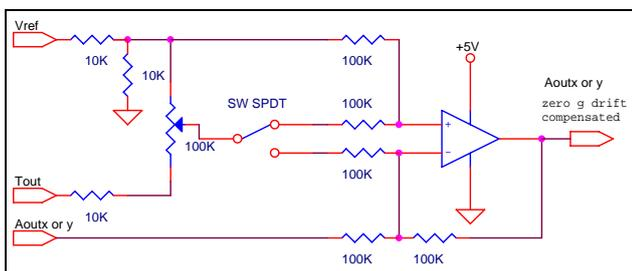
Figure 7: Zero g Offset Temperature Compensation Circuit
