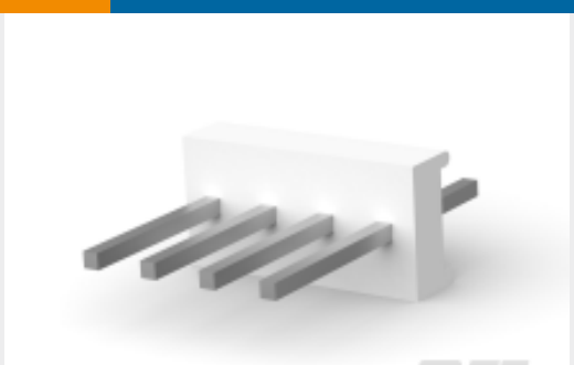
TE Part #3-641126-6 PCB Header: Polyester, Vertical, Unshrouded, No Mating Alignment
