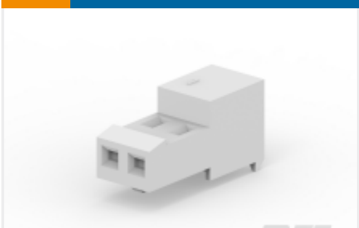
TE Part #3-640442-7 MTA Receptacle: Nylon, Tin Plated, 2.54 mm
