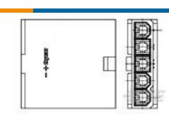
TE Part #1586103-3 3P PLUG VAL-U-LOK SR FH V2
