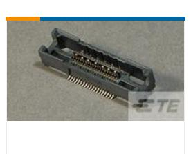
TE Part #5767096-8 MICT,REC,038,ASY,.025,TAPE,CAP
