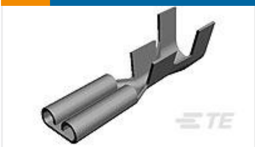
TE Part #160484-4 110 FASTON,REC.,20-17 AWG,BR
