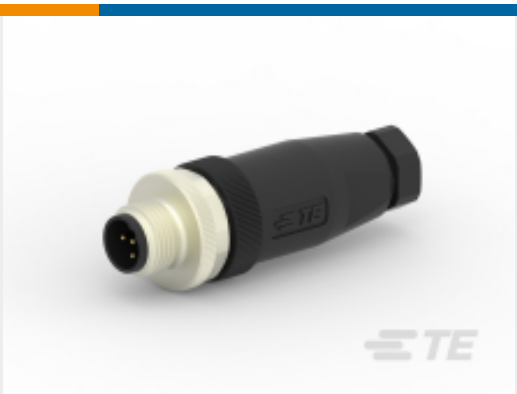
TE Part #T4111401051-000 M12,MALE,STRAIGHT,B CODE,5P, PG7,GOLD
