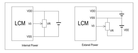
VDD-V0: LCD Driving Voltage
