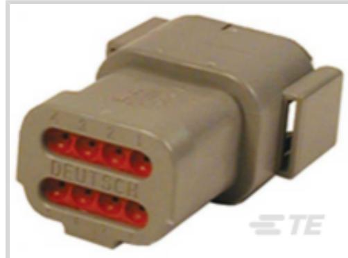
Connector System: **Wire-to-Wire**Number of Positions: **8**Connector & Housing Type: **Housing for Male Terminals**Centerline (Pitch): **4.19 mm [.165 in]**Sealable: **Yes**[All DEUTSCH DTM Housings \(109\)](#)
