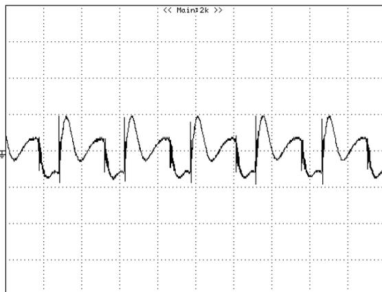
**Figure 12:** Output voltage ripple at nominal input voltage ( $v_{in}=48v$ ) and rated load current ( $I_o=15A$ ) (50 mV/div, 1us/div). Load capacitance:  $1\mu F$  ceramic capacitor and  $100\mu F$  tantalum capacitor. Bandwidth: 20 MHz. Scope measurements should be made using a BNC cable (length shorter than 20 inches). Position the load between 51 mm to 76 mm (2 inches to 3 inches) from the module
