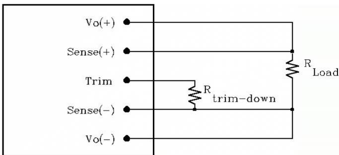
**Figure 16:** Circuit configuration for trim-down (decrease output voltage)
