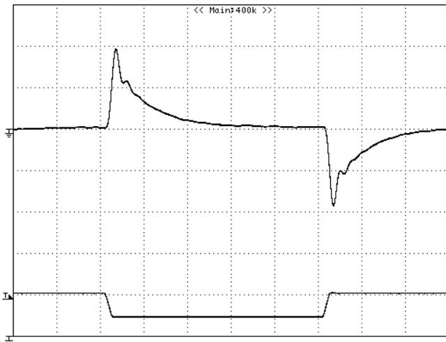
**Figure 6:** Output voltage response to step-change in load current (50%-25%-50% of  $I_{o, max}$ ;  $di/dt = 0.1A/\mu s$ ;  $V_{in}$  is 24v). Load cap: 10 $\mu F$  tantalum capacitor and 1 $\mu F$  ceramic capacitor. Top Trace:  $V_{out}$  (50mV/div, 200us/div), Bottom Trace:  $I_{out}$  (5A/div). Scope measurement should be made using a BNC cable (length shorter than 20 inches). Position the load between 51 mm to 76 mm (2 inches to 3 inches) from the module.
