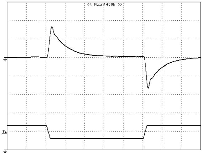
**Figure 7:** Output voltage response to step-change in load current (50%-25%-50% of  $I_{o, max}$ ;  $di/dt = 0.1A/\mu s$ ;  $V_{in}$  is 48v). Load cap: 10 $\mu F$  tantalum capacitor and 1 $\mu F$  ceramic capacitor. Top Trace:  $V_{out}$  (50mV/div, 200us/div), Bottom Trace:  $I_{out}$  (5A/div). Scope measurement should be made using a BNC cable (length shorter than 20 inches). Position the load between 51 mm to 76 mm (2 inches to 3 inches) from the module.
