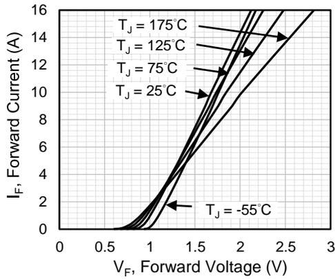
Fig.1 Forward Characteristics
