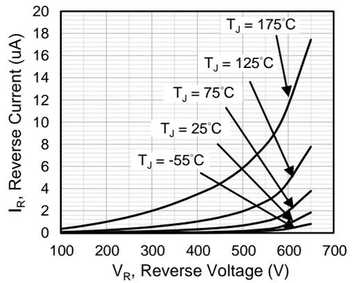
Fig.2 Reverse Characteristics
