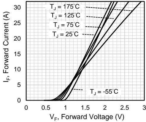
Fig.1 Forward Characteristics
