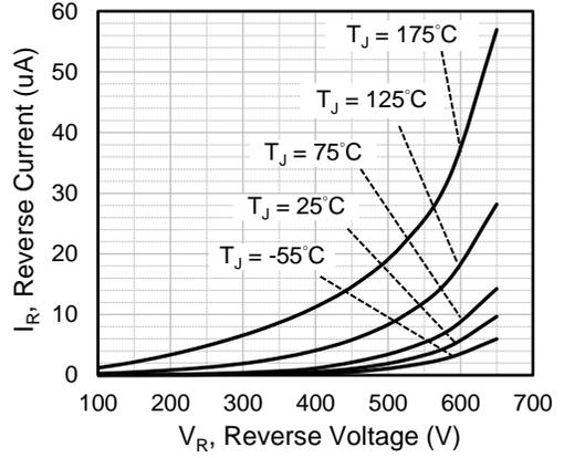
Fig.2 Reverse Characteristics
