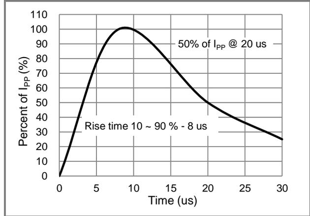
Fig.2 Pulse Waveform
