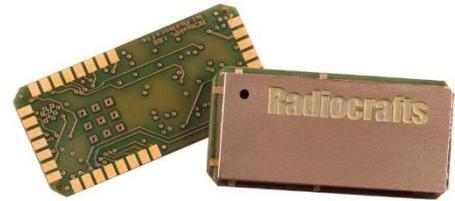
The module includes ICI, the intelligent C-programmable I/O, along with all necessary drivers and the operating system. ICI allows the user to program his own intelligent sensor/actuator interface, or any other application with minimal effort. The programming capability of the module makes it possible to interface to any sensor/actuator or combination of sensors/actuators. Thereby removing the need for an additional MCU to reduce overall cost and power consumption.
