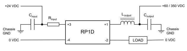
$C_{input}$  = 1 nF 2 kV (Y2 class, ceramic disc)  $R_{input}$  = 10  $\Omega$  (0.25 W)  $L_{\text{output}}$  = ferrite core + 4 turns  $C_{\text{output}}$  = 1 nF 2 kV (Y2 class, ceramic disc)
