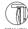
DETAIL VIEW VH1, VH3 & VH5 HOLE PLUGS (No wing serrations for ease of removal)
