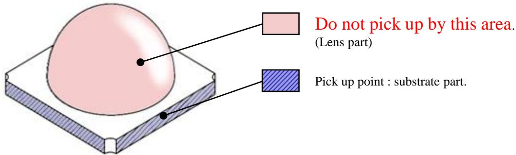
13. Low hardness resin is used for lens. Please avoid overload to the surface of lens which might cause chip-outs, encapsulant delamination, and deformation, nicks, wire disconnection and decreasing reliability.
