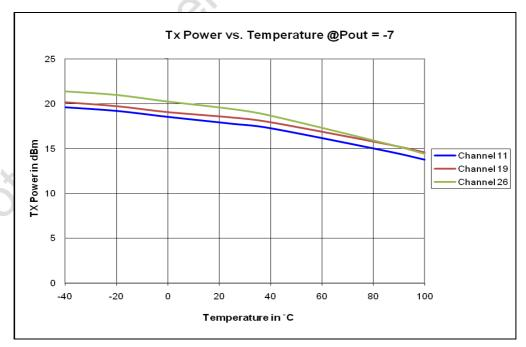
Figure 6. TX Power vs. Temperature
