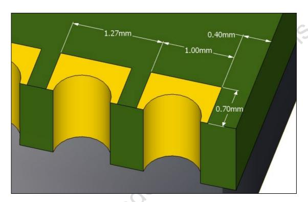
Figure 11. Typical pad dimensions
