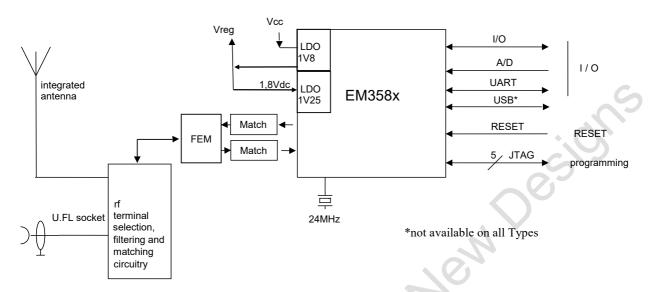
Figure 2. Hardware Diagram
