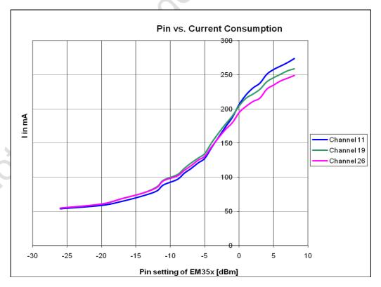
Figure 4. Module Current vs. Power Setting
