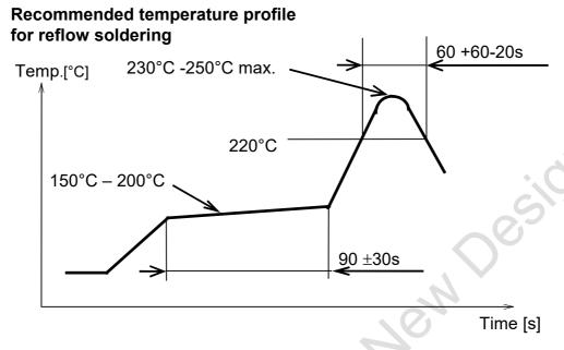
Figure 8. Recommended Reflow Profile
