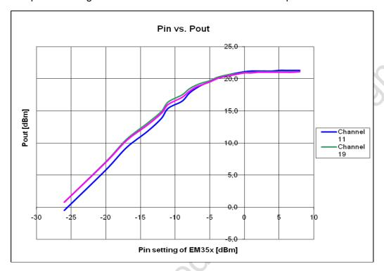
Figure 3. Output Power vs. Power Setting
