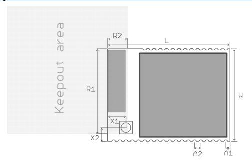
Figure 7. ETRX3 Physical Dimensions
