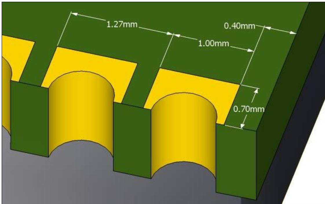
Figure 8. Typical pad dimensions
