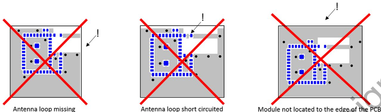
Figure 4.4. Poor Layout Designs for the BGX13S
