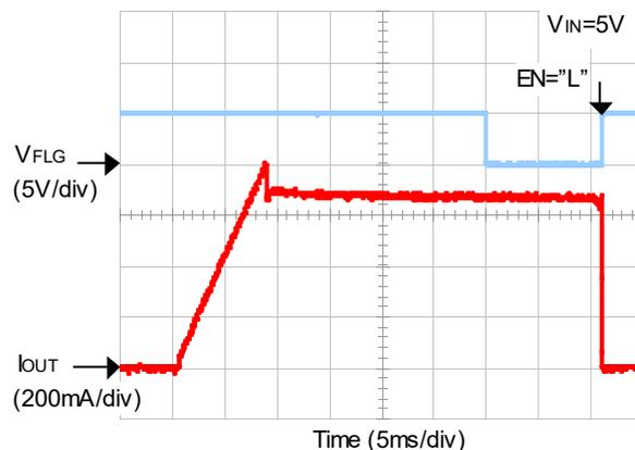
21) Overcurrent Response with Ramped Load
