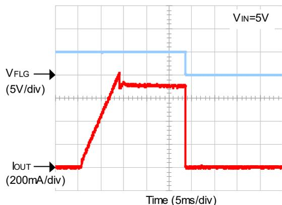
20) Overcurrent Response with Ramped Load
