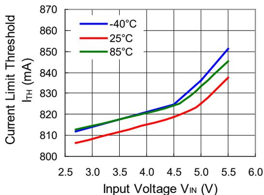
12) Current Limit Threshold vs. Input Voltage (004A)
