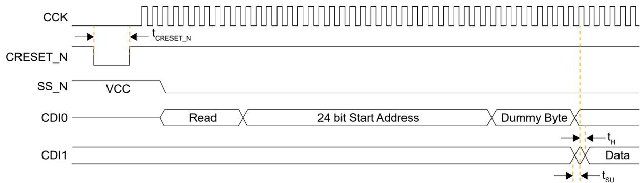
Figure 24: SPI Passive Mode (x1) Timing Sequence
