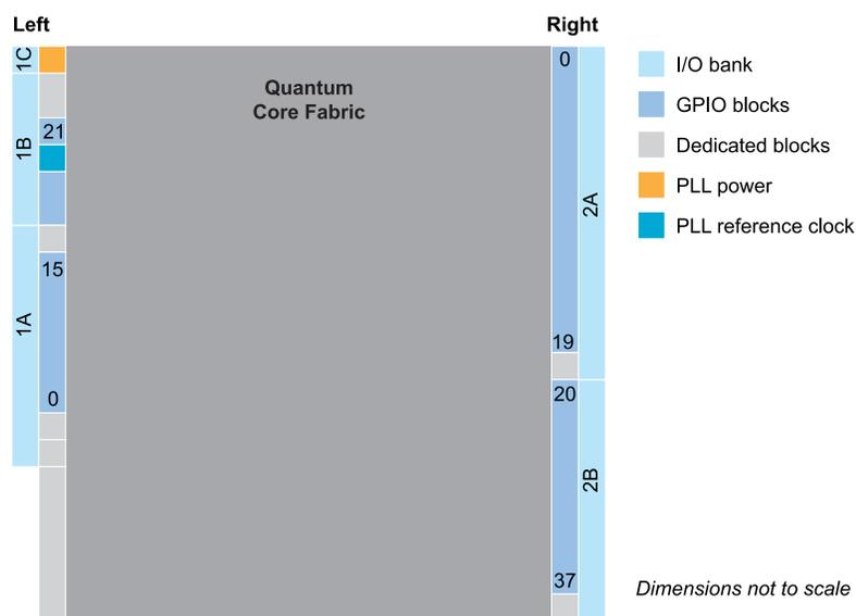
Figure 27: Floorplan Diagram for QFP144 Packages
